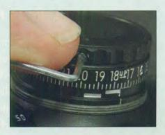
without raising your head completely off the stock. The magnification adjustment dial is deeply knurled and turns smoothly with just the right degree of tension to prevent accidental turning. It turns clockwise from lowest to highest magnification.
