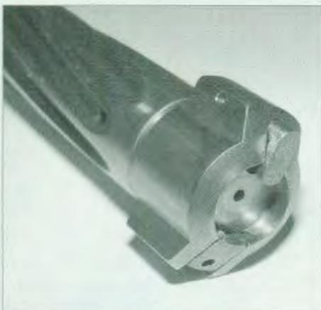
*Kelbly passive ejector (shown extended) installed in my Teddy action.*
